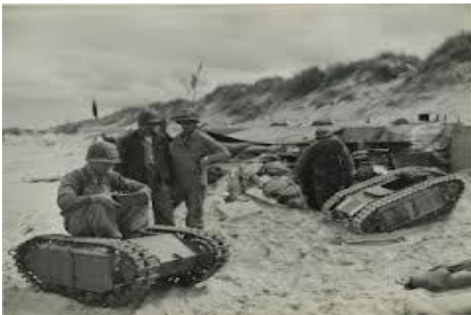
Figure 3. The miniature robot “Goliath”
